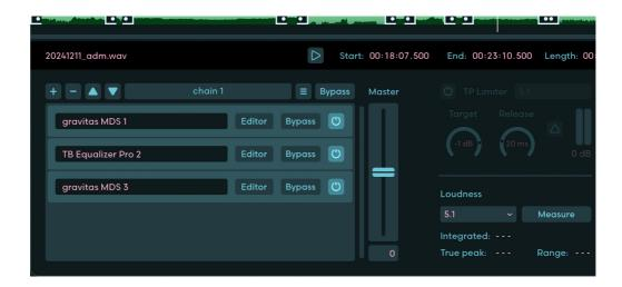
You can process a clip with plug-ins in its master channel. For Dolby Atmos content, there are OBAM plug-ins, which can process the entire Dolby Atmos mix with up to 128 channels And for stereo files, you can use your full arsenal of VST3 plug-ins. If there is any problem with an OBAM plug-in and it cannot be loaded, or if it crashes, a small text file is stored next to it which can help us diagnose the problem.
