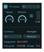
Here, you can adjust the target limit that should not be crossed, the release time and the format, which in most cases should stay at 5.1 since this usually is the format used for loudness measurement by the streaming services.
