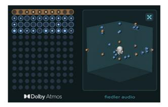
The channel meters and the 3D-View in the lower right corner show you what is currently going on at the playback position. The round channel meters in the lower right corner not only show the volume in each channel but also indicate the kind of channel that it is. Bed channels are shown in yellow while dynamic objects appear in blue.
