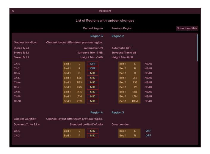
Each transition is displayed in two columns. The left shows the settings in the second region of the transition and the right column shows the settings of the first region of the transition. The differences are marked in red, just like the channel list in the Editor.
