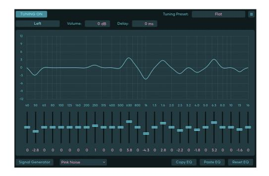
To the right of the Routing section, you'll find the Tuning section where you can set a volume, a delay time and an EQ curve for each and every channel, except for the headphones. By default, this section is turned off for performance reasons, but if you need to use it for your speaker calibration, you can switch it on and start tweaking.
