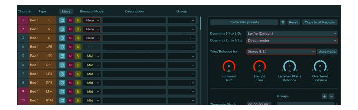
If there are differences in the Trim or Balance settings of any format, the format selector is marked in red. To see which trim/balance settings are actually different you'll have to check each format
