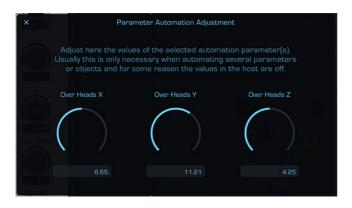
When the objects of the automated sources are spread out in such a way that the range of the possible automation seems to be insufficient, like hitting an "invisible wall", the small Q button comes to the rescue. Opening it you have access to the actual automation parameters and you can correct them there, without changing object positions in space.
