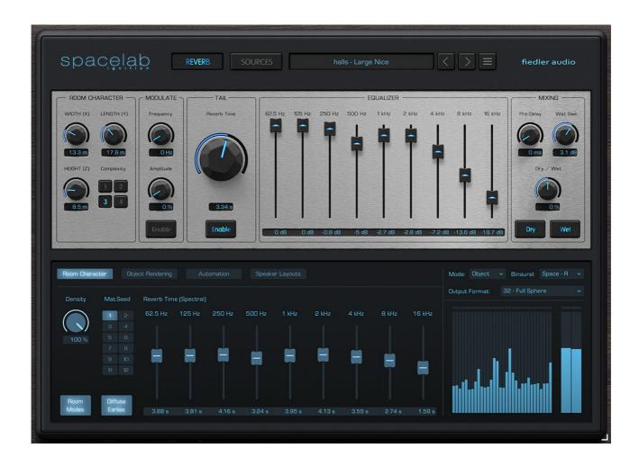
The reverb view is split into two parts. The top part in brushed metal design contains the essential reverb parameters and the bottom part contains four tabs with different parameters and editors plus the output section where you can select the formats to which Spacelab will render everything. The four tabs contain parameters for finetuning the reverb, object rendering, dynamic automation and the speaker layout editor.
