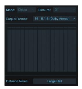
In a Dolby Atmos Composer session Spacelab is automatically connected to the Composer. The default Output Format is "16 –9.1.6 (Dolby Atmos)" which is routed to the Composite. This layout is located in the subfolder containing the layouts which should be used when working in Dolby Atmos. You can of course change the layout in the Composer at any time. Spacelab's own binaural rendering is not available when connected to the Dolby Atmos Composer.
