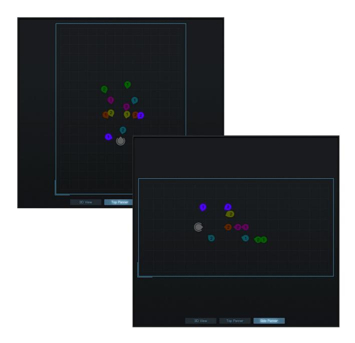
The Top Panner and the Side Panner are actually for panning by dragging sources and objects around. The background contains a grid where each square of it represents a square meter in the room.
