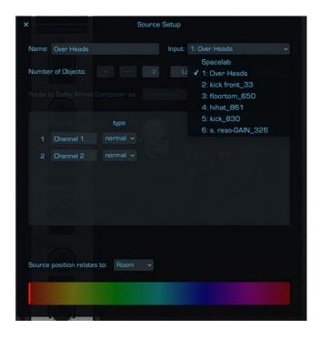
With the Input dropdown menu in the upper right corner of the dialog window you can choose between Spacelab's own plug-in input, labeled "Spacelab", and the available Beam plugins in your session.
