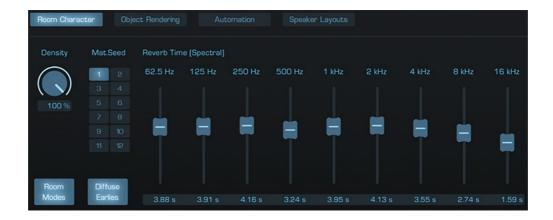
The Room Character tab contains further parameters for designing the overall sound of the reverb.
