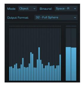
In the output section on the Reverb page you can see settings for an Output format and for Binaural. By default Binaural is set to off and the Output Format is set to Stereo Wide. If you intend to use Spacelab with multichannel formats you need to select the appropriate format from the Output Format dropdown to match the format of the track Spacelab sits on.
