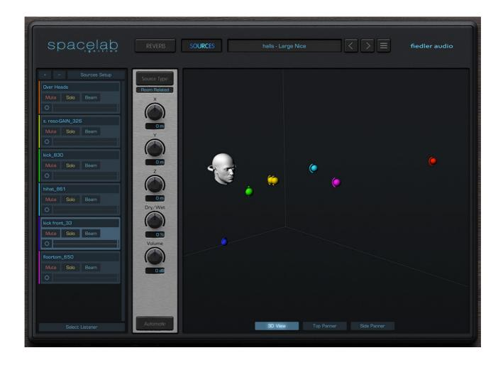
The sources page contains the list of sources (inputs) to Spacelab on the left, the control column right next to it and panner on the right side. Up to 24 objects and the listener can be moved around in the virtual room defined by the room dimensions set on the reverb page.
