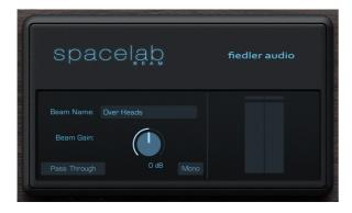
Spacelab Beam is the other plug-in which is installed together with Spacelab. With Beam you can send audio from anywhere in your session to Spacelab and thereby have up to 24 inputs in Spacelab Ignition even on stereo-only DAWs. This is achieved by circumventing the DAW's own mixing engine and sending the audio directly from Beam to Spacelab.
