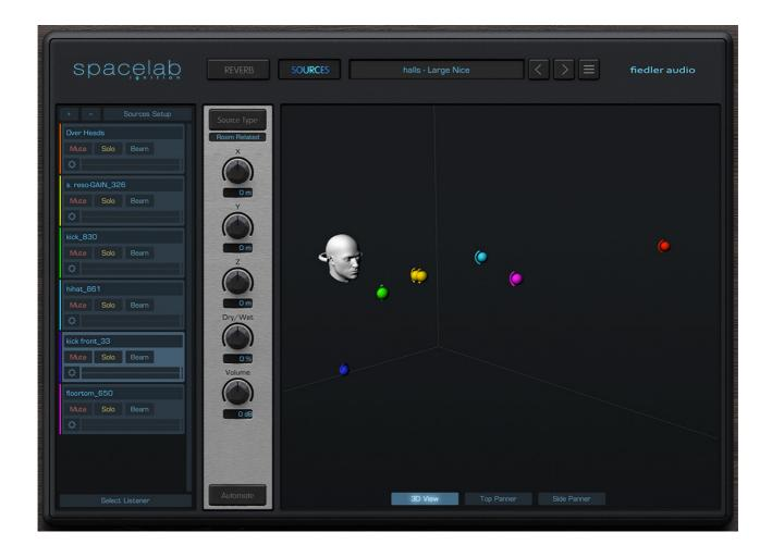
In Spacelab each incoming audio channel is treated as an object with a position inside a virtual room, in which all objects and the listener are positioned. The dimensions of this virtual room is set by the three knobs in the ROOM CHARACTER sub section on the Reverb page.
