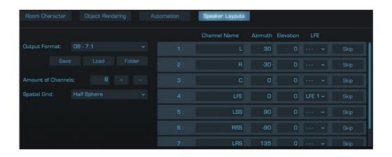
A speaker layout can contain between 1 and 256 speakers. On the left side in this tab you find the selector for the speaker layout presets. This selector is identical to the selector in the output section. When selecting a layout it is loaded as Output Format and can be monitored through your speakers or through headphones using the binauralizer.
