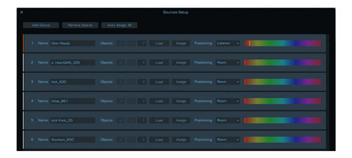
When clicking on the "Sources Setup" button on top of the sources list, the dialog window for batch configuration of your sources opens. There you find basically all the controls from the source configuration dialog but in a list form. You can change source names, configure number of objects and layout, set the source positioning mode and color. When clicking on the "Assign" button another dialog opens.
