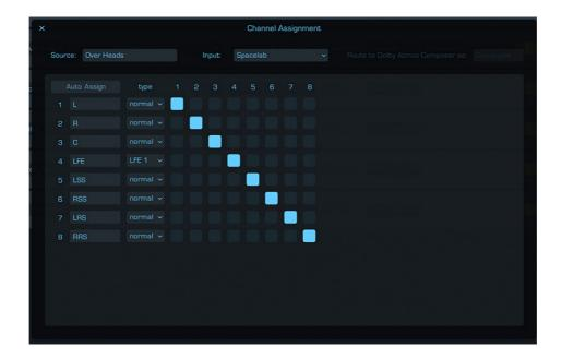
In this assignment dialog you find the same channel assignment matrix as in the source setup dialog. On top of it you can change the source name, select the input (either Spacelab or a Beam) and, in case the Dolby Atmos Composer is present, choose if the source shall be mixed to the Composite or be a bunch of dynamic objects.
