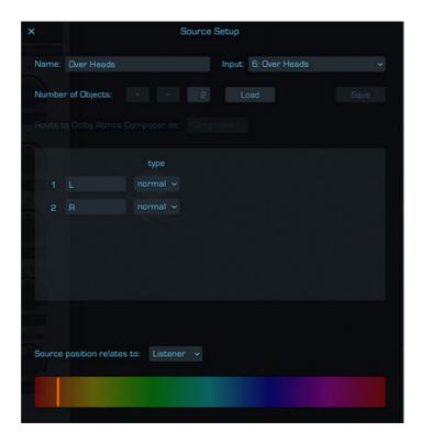
In the first line of the Source Setup dialog you can change the source name on the left, and on the right you can select the audio input for the source. By default the audio input is set to "Spacelab", meaning that the source receives its audio from Spacelab's own plug-in input. If Spacelab Beam plug-ins are present in the session you can see the list of them in the dropdown and select one as the source input.
