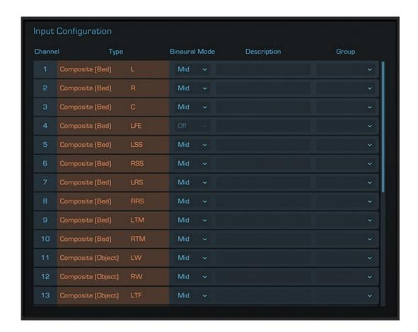
The second page is the Input Configuration list containing all channels in your Dolby Atmos mix. Composite channels are orange and dynamic objects are blue. On this page you can adjust various channel related parameters, such as Binaural Mode, Description and Group assignment.
