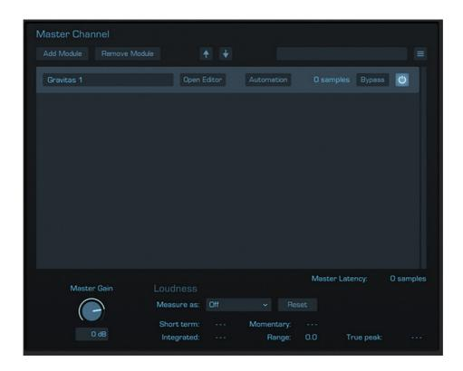
The Master Channel sits directly before the Dolby Atmos renderer, but after all the incoming connections have been mixed together. The channels of the mix pass through the module chain in the Master Channel and are then leveled by Master Gain. Master Gain by the way can be automated. After that, the mix goes into the Dolby Atmos renderer integrated into the Composer where the rest happens.
