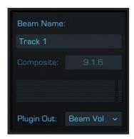
On the top of the output section you find the field for setting the name of the Beam. When instantiated Beam tries to retrieve the track name from the DAW, which is no problem in most cases. You can change it always to whatever you want and the change is communicated to the Composer.
