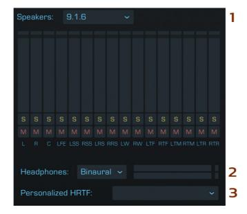
When instantiated on a multichannel track the Dolby Atmos Composer will set the appropriate speaker layout (1) if there is a match. Otherwise headphone monitoring is enabled (2) by default using the binaural setting. You can of course change both manually and you can also monitor both simultaneously.
