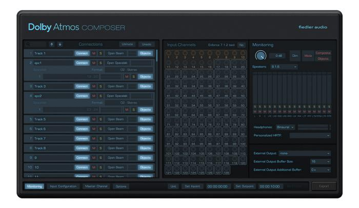
On the left side you'll find the list of incoming connections. Those can be Dolby Atmos Beam plug-ins or Spacelab plug-ins. Below this list are the four buttons giving you access to different pages on the right, the Monitoring section, the Input Configuration, the Master Channel and the Options page.
