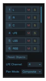
On the top of the input section you find the input channel list. In this list you can change the input names and mute or solo each of the input. Mute and solo are not just for monitoring purposes and their setting is stored with your session.
