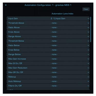
The image on the left shows that Input Gain from the first module is on Lane 2.
