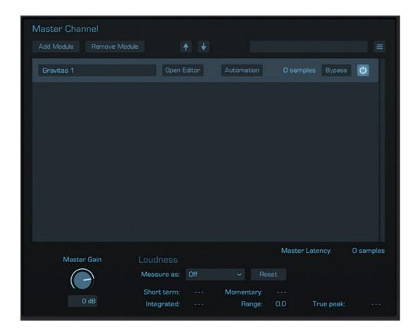
The third page is the Master Channel where you can load modules to process your Dolby Atmos mix as a whole. Below the list of the modules is the Master Gain knob and the Loudness measurement section.
