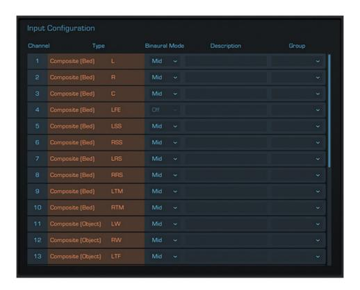
On the Input Configuration page you have access to the channel related features of Dolby Atmos. In the Binaural Mode column you can change how each channel is rendered when listening to your mix in binaural. Dolby Atmos offers 4 different options for each channel. "Off" means that no binaural processing is applied to the channel while the remaining three modes differ in the perceived distance.
